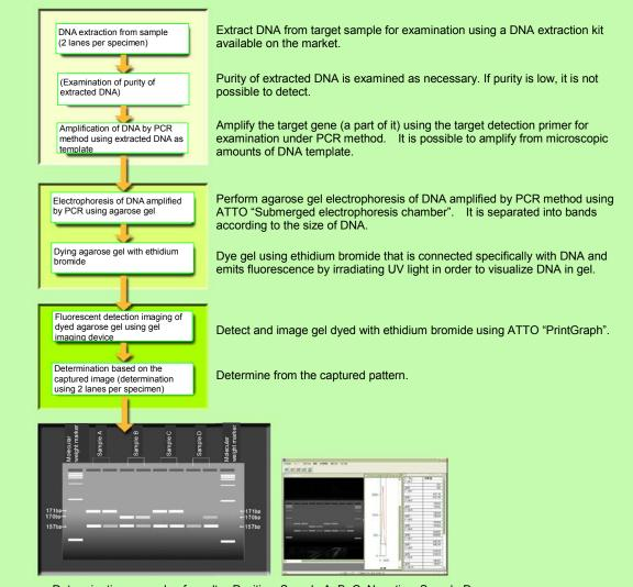
Determination example of result Positive: Sample A, B, C, Negative: Sample D Determination is made according to the presence of the target gene for examination (band) based on whether a band of marker DNA is detected or not.
